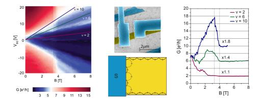
left: Conductance G as a function of magnetic field and gate voltage. middle: SEM picture of a typical device (top), quasiclassical illustration of chiral edge states along the sample border and an Andreev edge state along the N-S interface (bottom). right: conductance as a function of B for fixed filling factors  $\nu$ =2,6, and 10.
