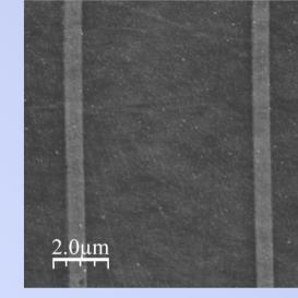
The (001) surface of a GaAs<sub>1-x</sub>N<sub>x</sub>/GaAs heterostructure (x=0.8%) was patterned with Ti wires (width w=500 nm) oriented at different angles (0°, 22.5°, 45°, 67.5° and 90°) with respect to the [110] crystallographic direction
