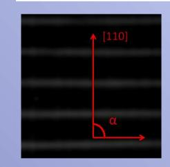
Polarization angle rotates with wire orientation: Light is polarized mainly in the direction perpendicular to the wires, as a consequence of different optical selection rules for the two polarizations
