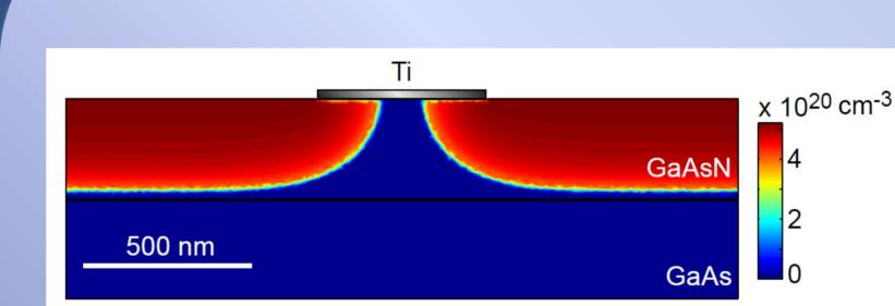
A simulation of hydrogen diffusion
