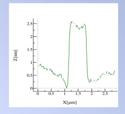
The topography map shows a protrusion of about 2 nm of GaAsN wires above hydrogenated barriers, which is due to strain modulation
