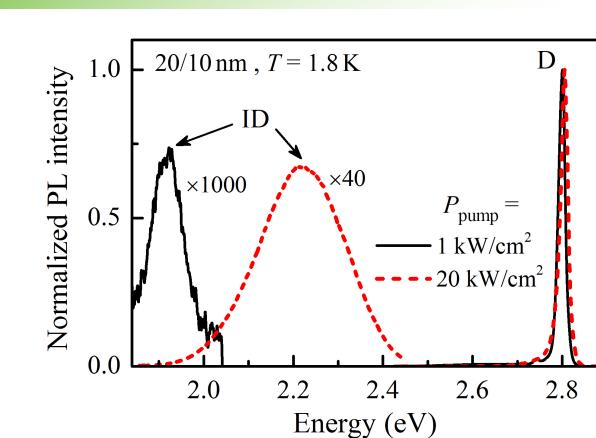
Spectral position and shape of indirect emission line strongly depend on excitation density due to internal electric fields
